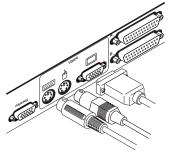
3. Locate the power cord that came with your APC KVM Switch unit. Plug it into the IEC power connector on the switch. Make sure that the APC KVM Switch power switch is off, then plug the other end of the power cord into an appropriate AC wall outlet. This outlet must be near the equipment and easily accessible to allow for unplugging prior to any servicing of the unit.
